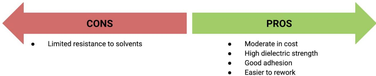
**Polyurethane** - This coating is known for excellent moisture and chemical resistance. However, this quality makes repair and reworking of the coated electronics a challenge. Polyurethane operates well in a wide temperature range and maintains flexibility at very low temperatures and is popular in industries like aerospace, automotive, and medical.
